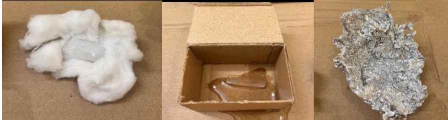
Figure 15 (d) Ice cube is slightly melted in cotton, partially melted in cardboard and completely melted in aluminium foil
