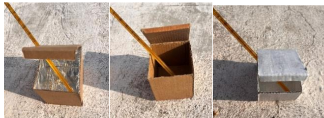
Figure 14 (b) Aluminum foil lined box measured as 37°C, Control box measured as 39 °C and white surface box measured as 36.5°C
