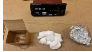
Figure 15 (c) After 30 mins the condition of the ice cube in different insulation materials
