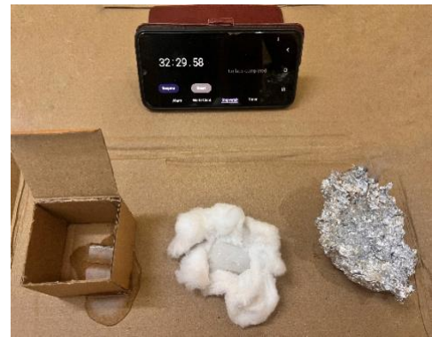
Figure 3.5 (c) After 30 mins the condition of the ice cube in different insulation materials
