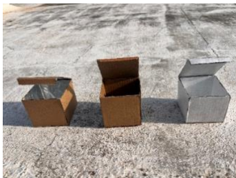
Figure 14 (a) Aluminum foil lined box, Control box measured as 41°C and white surface box are laid down under heat source
