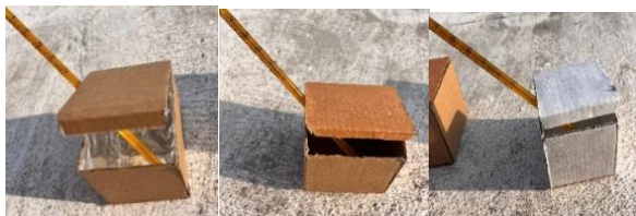
Figure (c) Aluminum foil lined box measured as 39°C, Control box measured as 40°C and white surface box measured as 38°C
