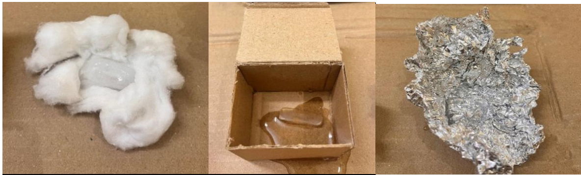
Figure 3.5 (d) ice cube is slightly melted in cotton, partially melted in cardboard and completely melted in aluminium foil
